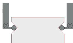
SLOTS AND RECESSES OUTSIDE CONTROLLO GUIDE A "V" ESTERNE
